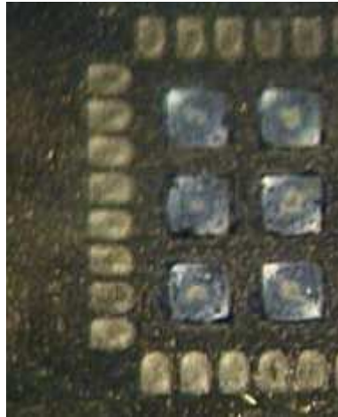
Figure 22 Base plate shows some wear due to socket
