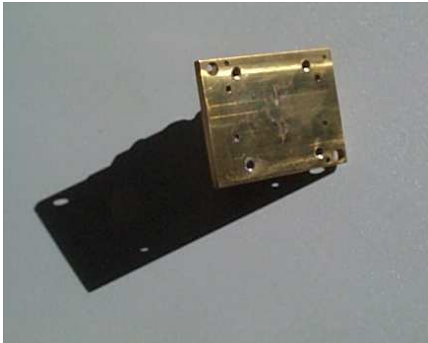
Figure 2 Kapton CSP socket mounting plate example
