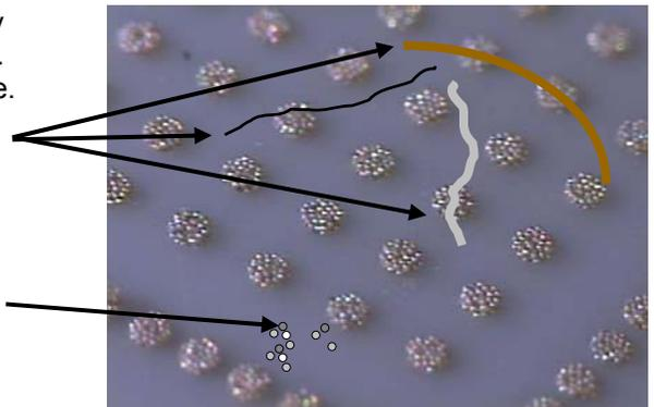
**Solder residue and oxide migration** – The amount of transfer may vary by the type of device and type of solder and it may build up on the Contact Set tips over high numbers of device insertions and cause an increase in contact resistance. The Contact Set tips may be cleaned with a brush to remove residue and oxides. (Note: Since the Silmat® does not touch the device leads, it should not accumulate solder residue and should not need to be cleaned.)
